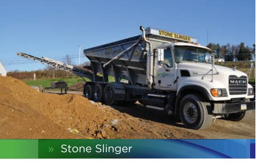
Ecotech's Stone Slinger precisely places material from up to 100 feet away, with a 180° radius. Our conveyor system is the fastest way to spread aggregate, soil and sand on any job site.
